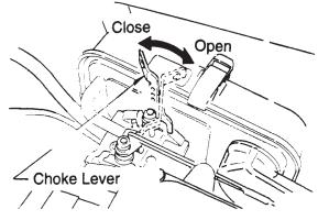
Figure 9. Choke Lever
